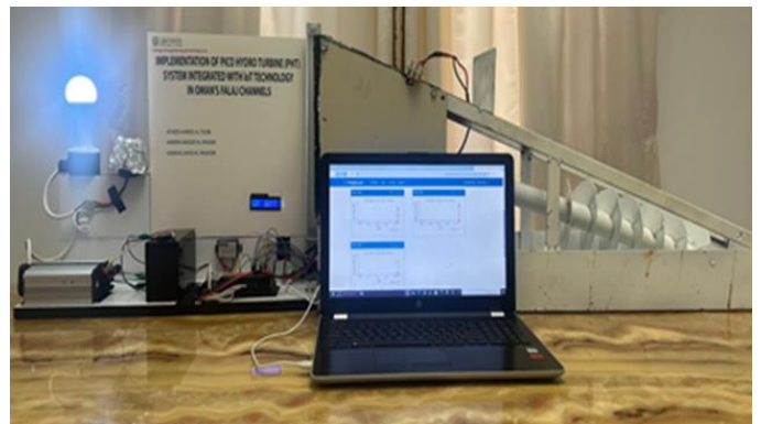
Figure 9: PHT Prototype with Arduino – IoT Set up
