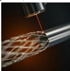
Figure 16 Laser Cutting process of stent.
