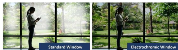
Fig. 6 Electrochromic glass in indoor environment. Source: https://www.energy.gov/eere/buildings/articles/better-windows-better-outcomes-how-electrochromics-improve-health .
